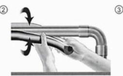
Open pre-slit Armaflex and snap onto pipe (release paper is still protecting the self-adhesive strip).
