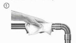
Clean all dust, dirt, oil from pipework where necessary. Install Armaflex when ambient temperature is between +4 and +38°C
