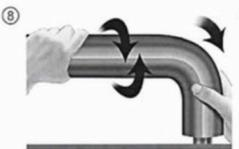
Using a circular motion, push the Armaflex around bends. Do not pull the insulation. On tight radius bends use mitre-cut sections.
