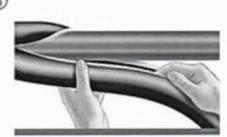
Adjust fitted Armaflex to ensure slit is easily accessible.
