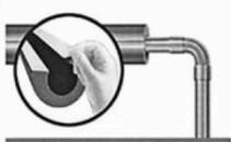
Locate the end of the yellow release film for the self-seal strip.
