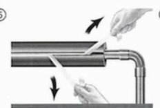
Remove the yellow protection plastic strip on both sides by drawing it away from the insulation.
