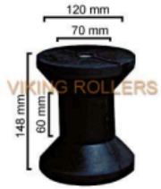
91241 = 6" Jumbo Roller Black 17mm bore. dia. : 70 / 120mm length : 60 / 148mm
