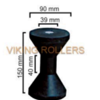
91240 = 6" Deep "V" Roller Black 17mm bore. dia. : 39 / 90mm length : 40 / 150mm
